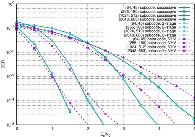
Fig. 4. Systematic polar subcodes [4] versus systematic Arikan polar codes.
