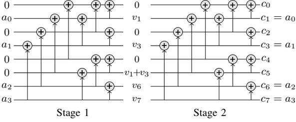
Fig. 1. The two-stage systematic encoder for a polar subcode
