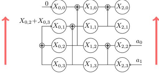
Fig. 2. The successive systematic encoder for a polar subcode
