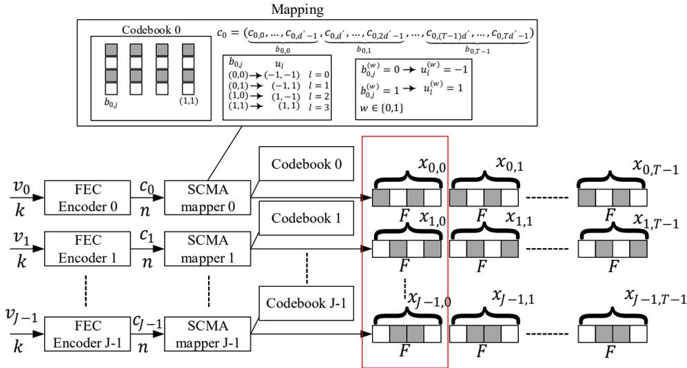
Fig. 1. SCMA transmitters with  $M = 4$ ,  $F = 4$ ,  $d = 2$
