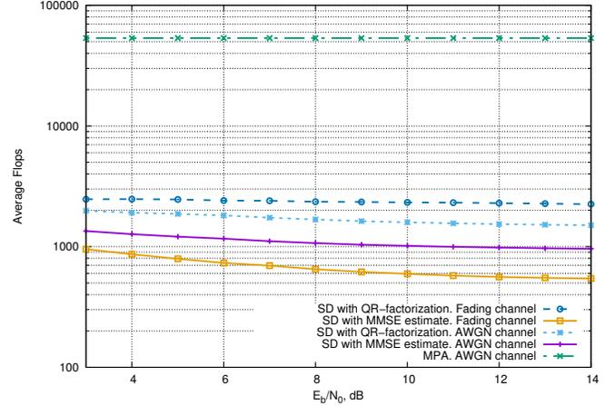
Fig. 5. Average flops of uncoded  $4 \times 6$  SCMA
