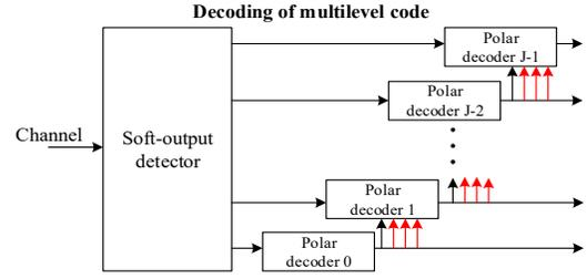
Fig. 4. Joint list decoding scheme
